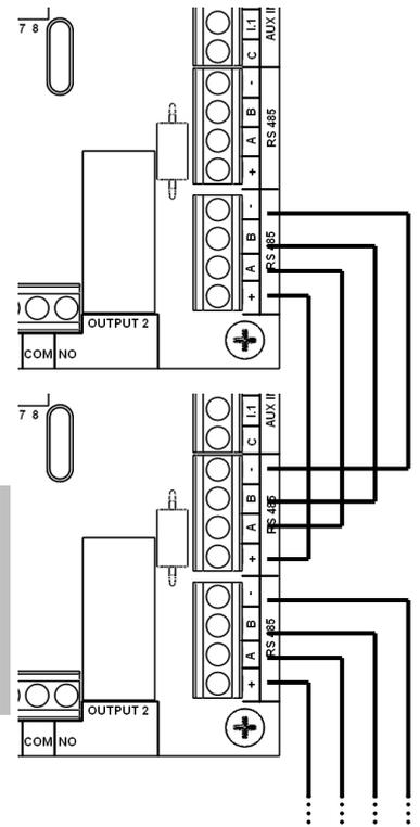
**CAUTION:** after connecting the devices to one another, they should be assigned an individual number to identify their address in the serial bus. Each device must be assigned a different number; otherwise, if several devices have the same address, the serial communication will overlap with loss of transmitted data.
