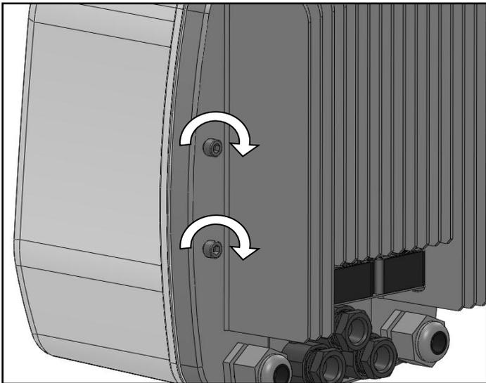
3) Pre-assemble the fixing screws on the rear side of Nettuno, leaving a space of at least 3 mm under the screws.
