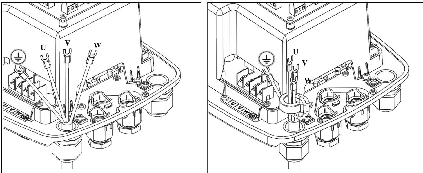
Connect the earthing wire to the corresponding terminal. Then proceed with the connection of the device power wires to the terminal board marked with the letters U, V, W as shown in the image below.
