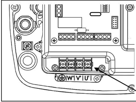
The recommended cable section is 2.5mm<sup>2</sup> for cable lengths from 2 to 30 metres. Longer cables, though admissible, have not been tested according to the EMI/RFI standards and must be evaluated by the manufacturer.
