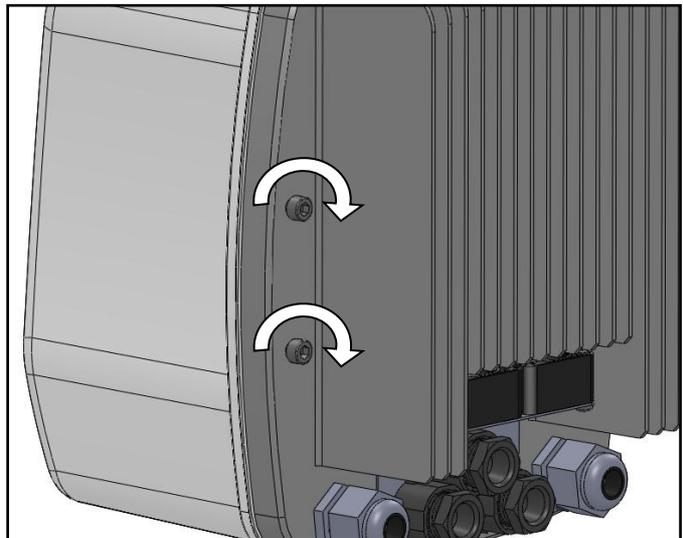
2) Pre-assemble the fixing screws on the rear side of *Nettuno*, leaving a space of at least 3mm under the screw heads.
