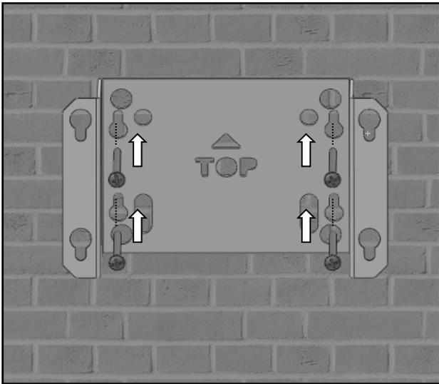
1) Fix the bracket to the wall by means of the 4 screws supplied. Check to ensure correct horizontal alignment.
