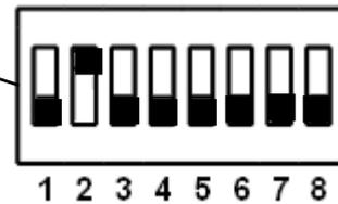
**⚠ The serial address value set via the dip switch on the I/O board must subsequently be entered in the software of each device on initial activation.**
