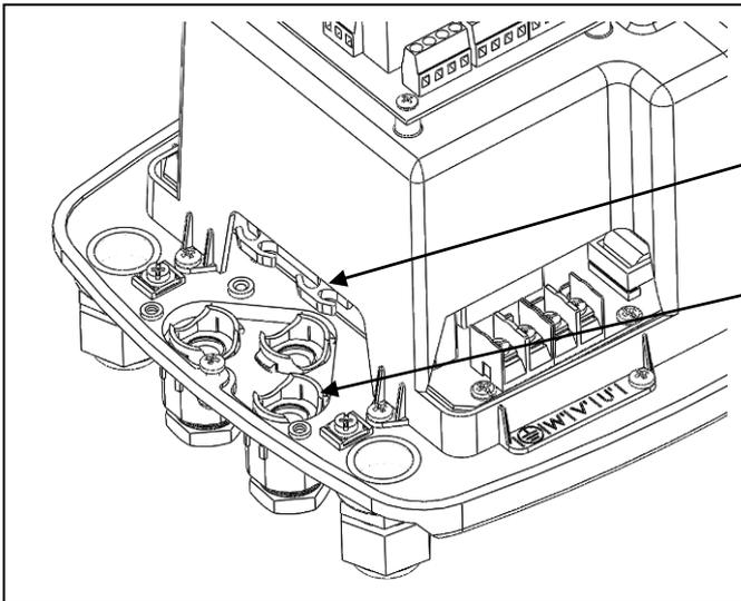
Insert the cables of the auxiliary devices via the central cable clamps in plastic. Use the relative cable guides to keep wiring tidy.
