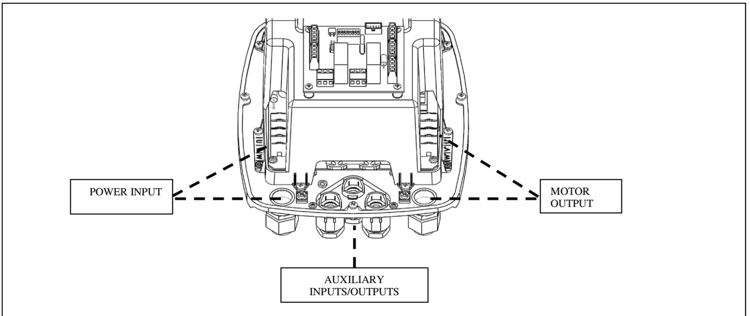
The metal plates located in the vicinity of the cable clamps can be used to connect the shielding of the cables and thus ensure correct continuity of the shielding itself with the heat sink.
