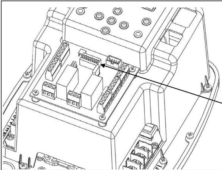
All devices are supplied with the address set to "1" as a factory setting, and therefore set up for use as a single unit. If used in a serial connection, a different address must be set for each connected inverter.
